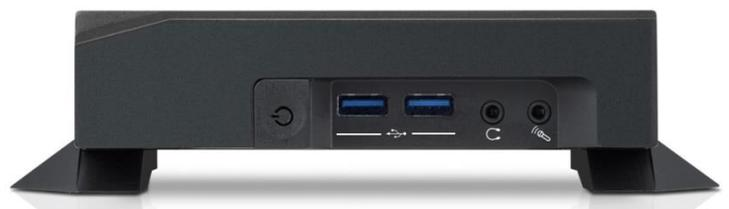
(Chassis with desk stand installed, horizontal operating mode)
