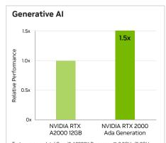
Tests run on an Intel Core i9-12900K Processor @ 3.2GHz (5.2GHz Turbo), 64GB RAM, Windows 11 Enterprise x64, Stable Diffusion WebUI v1.6.0, NVIDIA Driver 550.76. Average relative speedup for 512x512 and 1024x1024 image generation. Performance based on pre-release build, subject to change.
